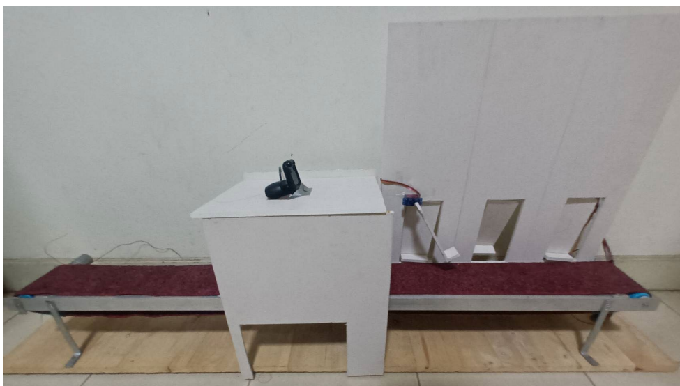
Figure 3. A prototype of Mango Grading Machine.
