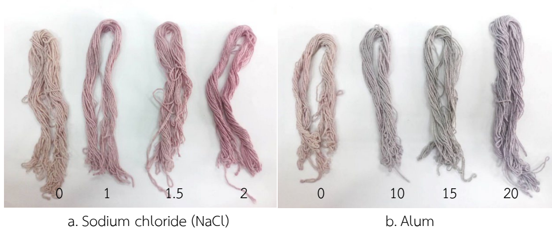
Figure 2. Yarn dyeing results with different concentrations of dye fixing agent and Mordant, respectively.
