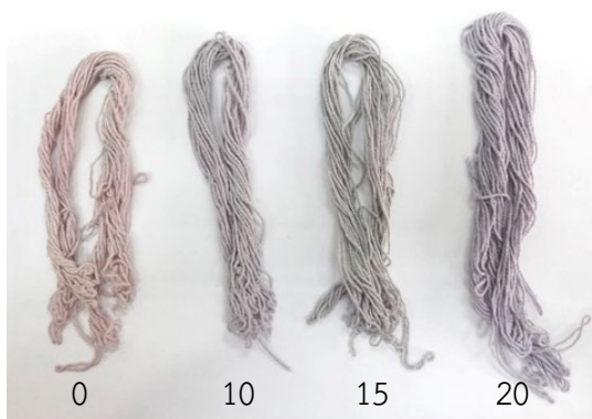
Figure 4. Yarn dyeing results with Makiang and Mordant extracts at concentrations of 0, 10, 15 and 20, respectively.
