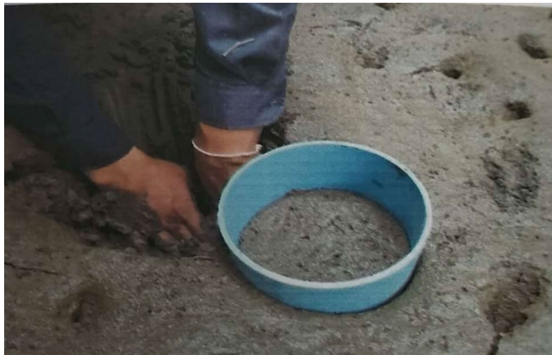
Figure 3. Bringing up the soil sampling cylinder Mangrove Forest Area, Sirinath Rajini Mangrove Ecosystem Education Center, Pak Nam Pran Subdistrict, Pran District Prajap Si Ri Khan Province.
